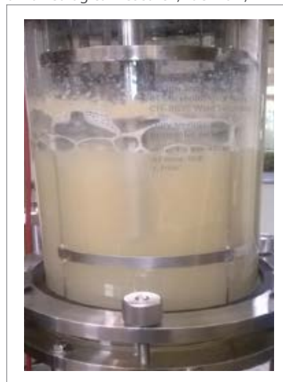
Scale up of the process for Xanthan gum in laboratory scale bioreactor
