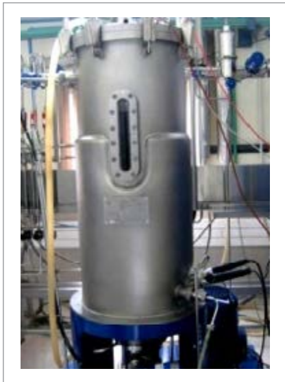
Fermentative biohydrogen production by C5 sugar utilizing Enterobacter cloacae DT-1 strain (isolated by TERI) from lignocellulosic biomass sugar (second generation feedstock) in 150 litre pilot scale bioreactor (100 litre working volume), through dark fermentation route
